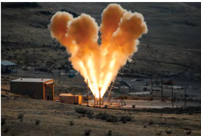
Static firing of the Orion escape rocket.
